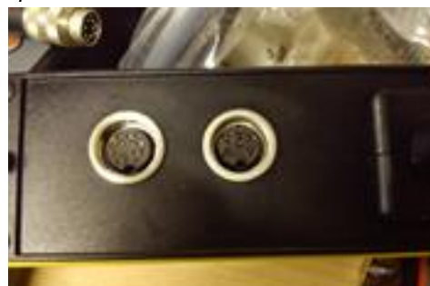
Photo 1b. Version with goggles. 5-pin socket for data transfer to a PC and 12-pin socket for goggles
