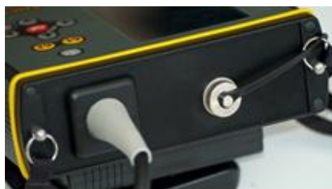
Photo 1a. Probe cable socket. PC transmission port
